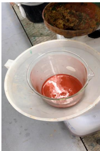
Figure D-1: Illustrates the procedure of collecting the non-contaminated heavy fluid at the end of the experiment [66].
