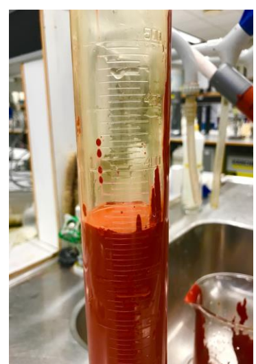
Figure D-1: Illustrates the procedure of collecting the non-contaminated heavy fluid at the end of the experiment [66].
