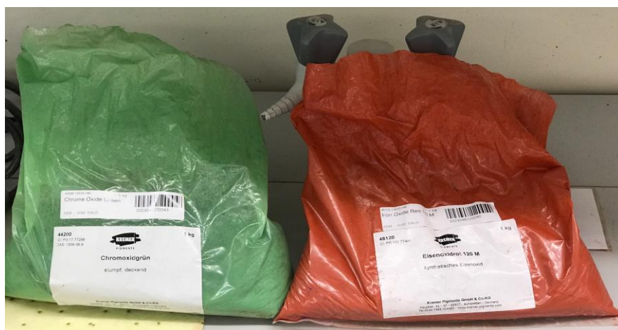
Figure C-4: Shows metal oxides that used as color indicator for the fluids [66].
