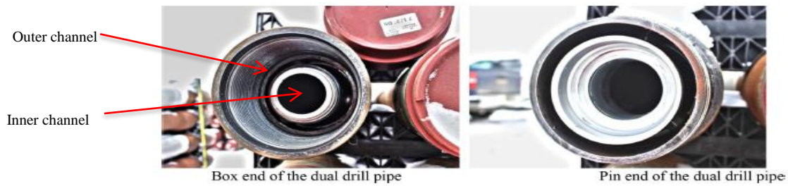
Figure 2-1: illustrates the inner geometry of a DDS [19].
