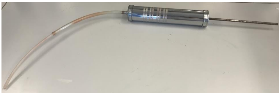
Figure C-6: A mechanical pump used for pumping the heavy fluid down into the well
