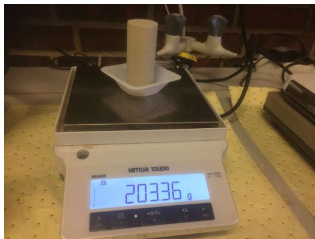
Figure 14. Illustration of weight measurement of the dry core of Bentheimer_1.
