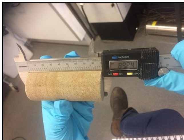
Figure 10. Illustration of measuring the dimensions of the core.
