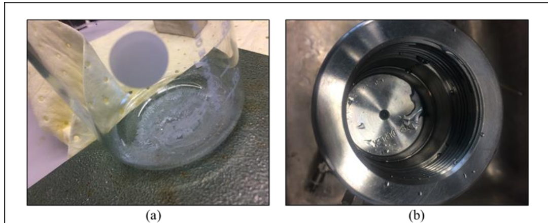
Figure 30. Quilon-L in distilled water: (a) after pouring the solution to filtration setup (b) solution left over inside piston cell.
