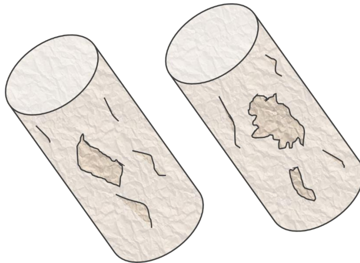
Figure 2.4 A schematic illustration of collapsed casings.
