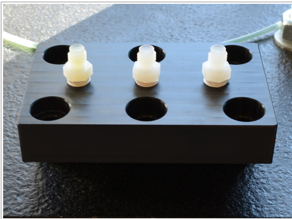
Figure 4.9: Filter module used in the POM cell.
