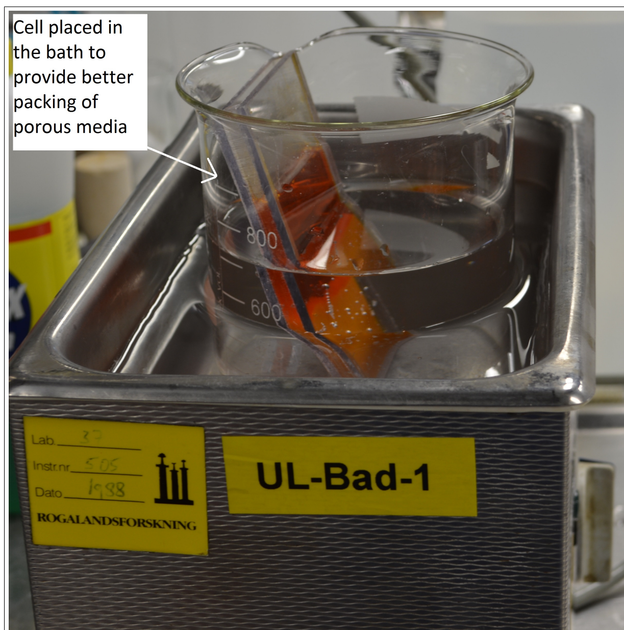
Figure 4.7: Polycarbonate cell in an ultrasonic bath.
