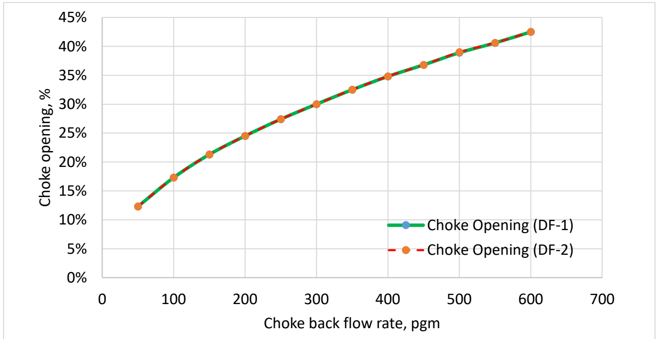
Figure 5.7: Choke opening during MPD connection case scenario for drilling fluids DF-1 and DF-2 at target ECD
