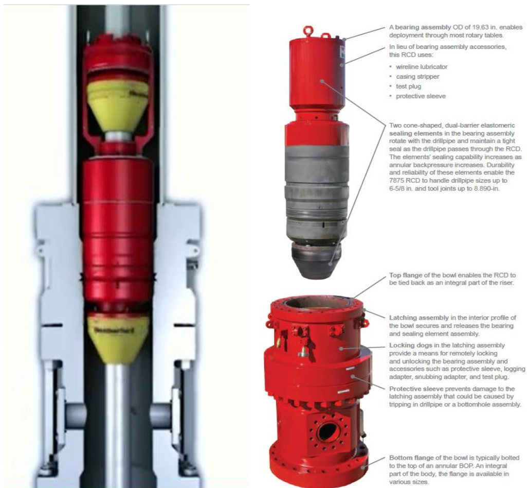
Figure 3.4: RCD part (Weatherford International Oil Field Services, u.d.)
