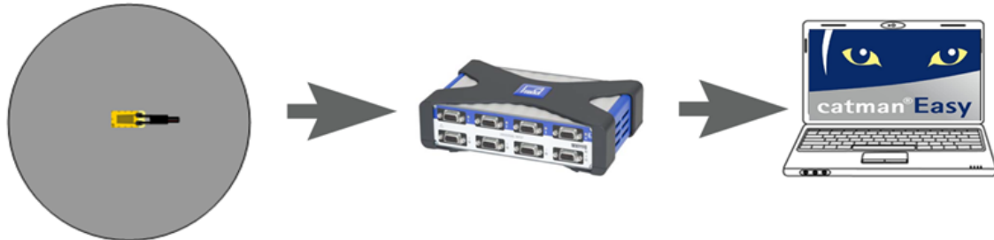
Figure 77: Steel plate with strain gauge, QuantumX and Computer with Catman 5.2 Software.
