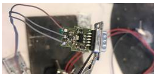
Figure 12: Strain gauge wires mounted to the SCM SG-120 adapter.
