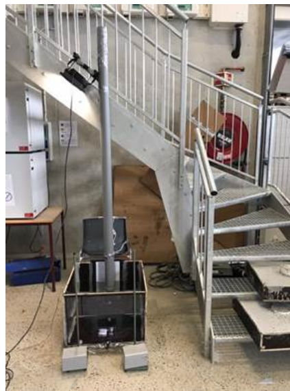
Figure 4: Test type 2 – Ball drop method.
