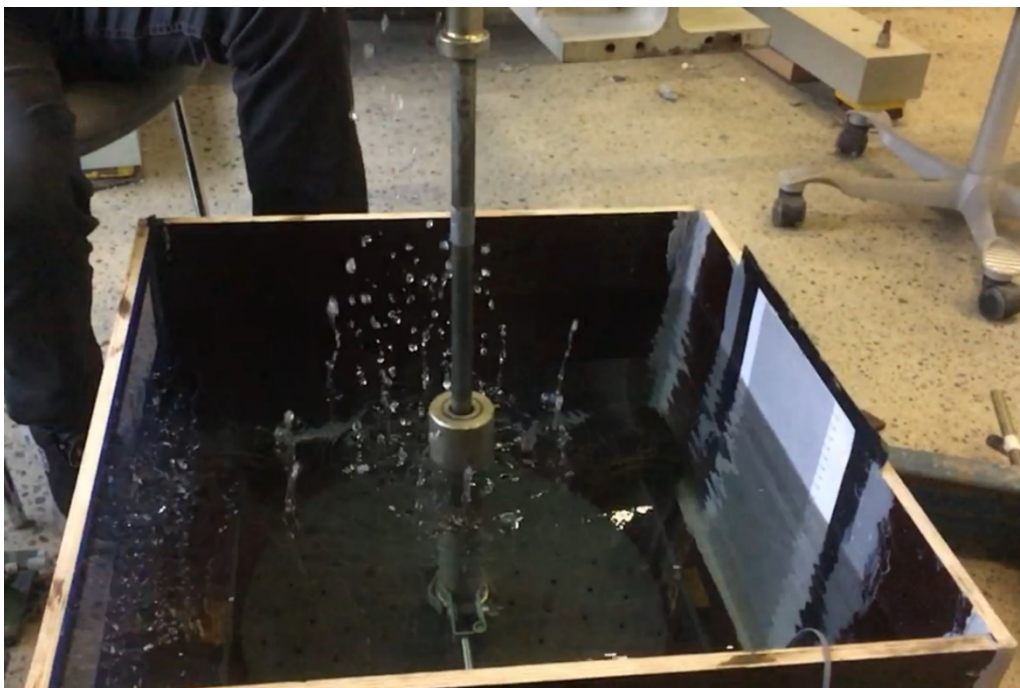
Figure 134: Image of the water Jet stream caused by impact on perforated plate.
