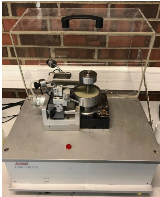
Figure 4-1: CMI tribometer at UiS
