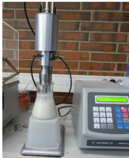
Sonication of BN + Lubricant
