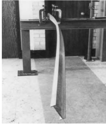
Figure 2.6: Lateral buckling of a cantilever beam [1]
