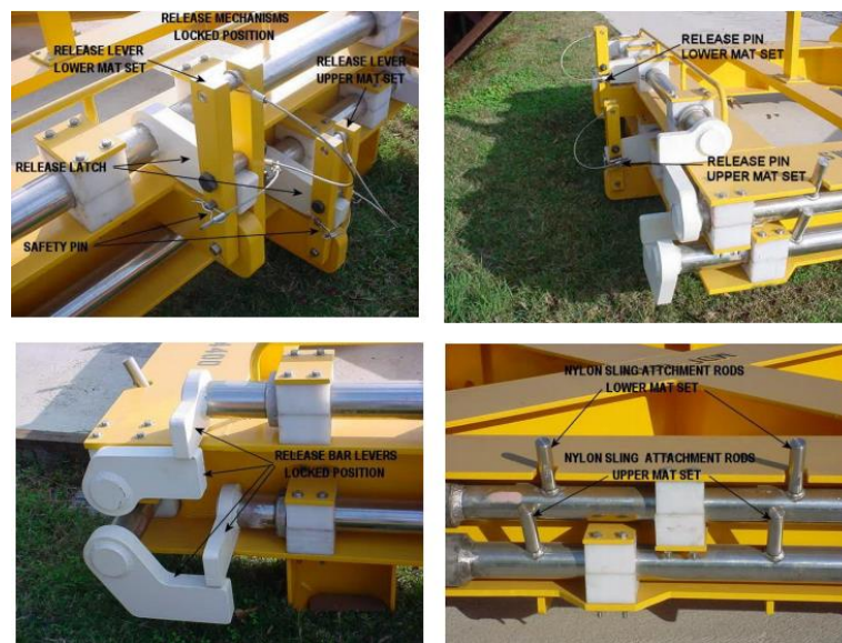
Figure 2.16: The mechanical releasing mechanism of the Submar frame (Submar.com)
