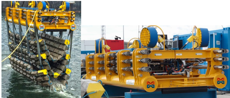
Figure 2.18: Left- MDS 3 on quayside, Right- MDS 3 during deployment of 3 concrete mattresses (offshoremm.com)
