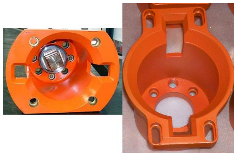
Figure 2.24: ROV bucket with (left) and without (right) stem (google.images.com)
