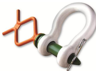
Figure 9.4: Green pin ROV shackle with tapered pin and fishtail-handle (vanbeest.nl)
