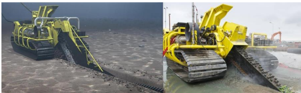
Figure 2.6: Illustration of mechanical trencher (seawayheavylifting.com.cy)
