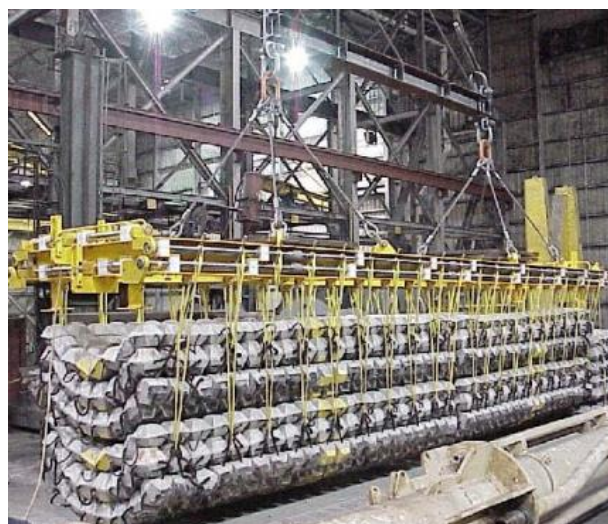
Figure 2.15: Multi-deployment frame provided by Submar ( Submar.com )
