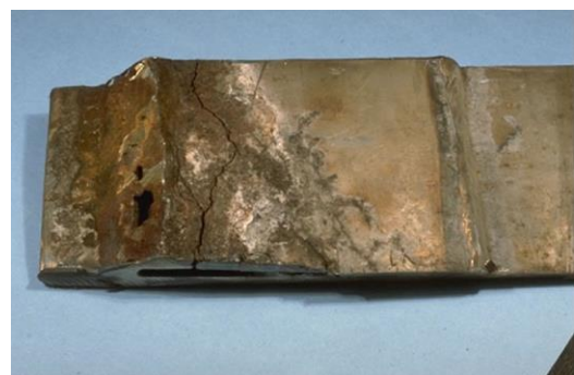
Figure 8: Example of Stress-Corrosion-Cracking(INSA, 2013b)
