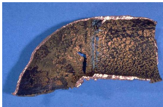
Figure 7: Example of Erosion-Corrosion(INSA, 2013a)
