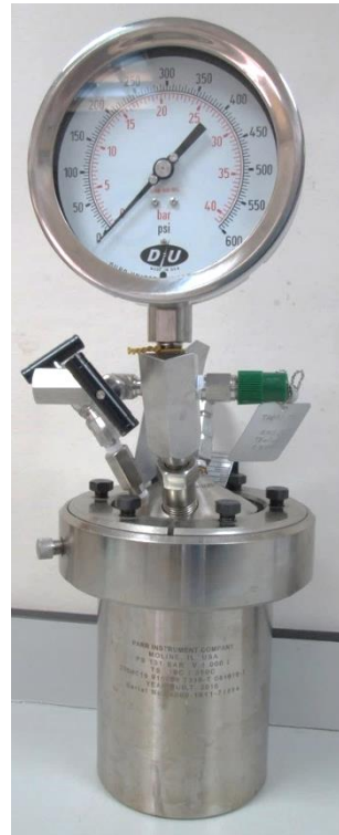
Figure 36: Assembled HPHT static Autoclave test equipment
