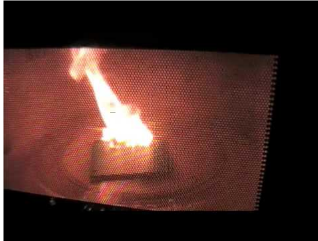
Figure 14: Arcing in a Microwave(Sagar, 2012)
