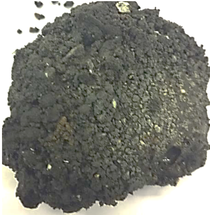
Figure 15: Hot spot as a result of thermal run-off (Egar, 2017)
