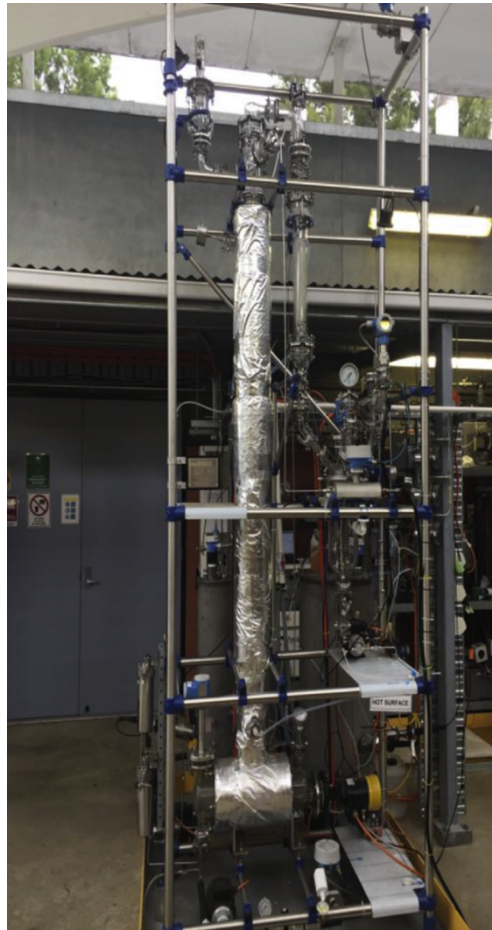
Figure 31: Distillation column used to separate MEG and water
