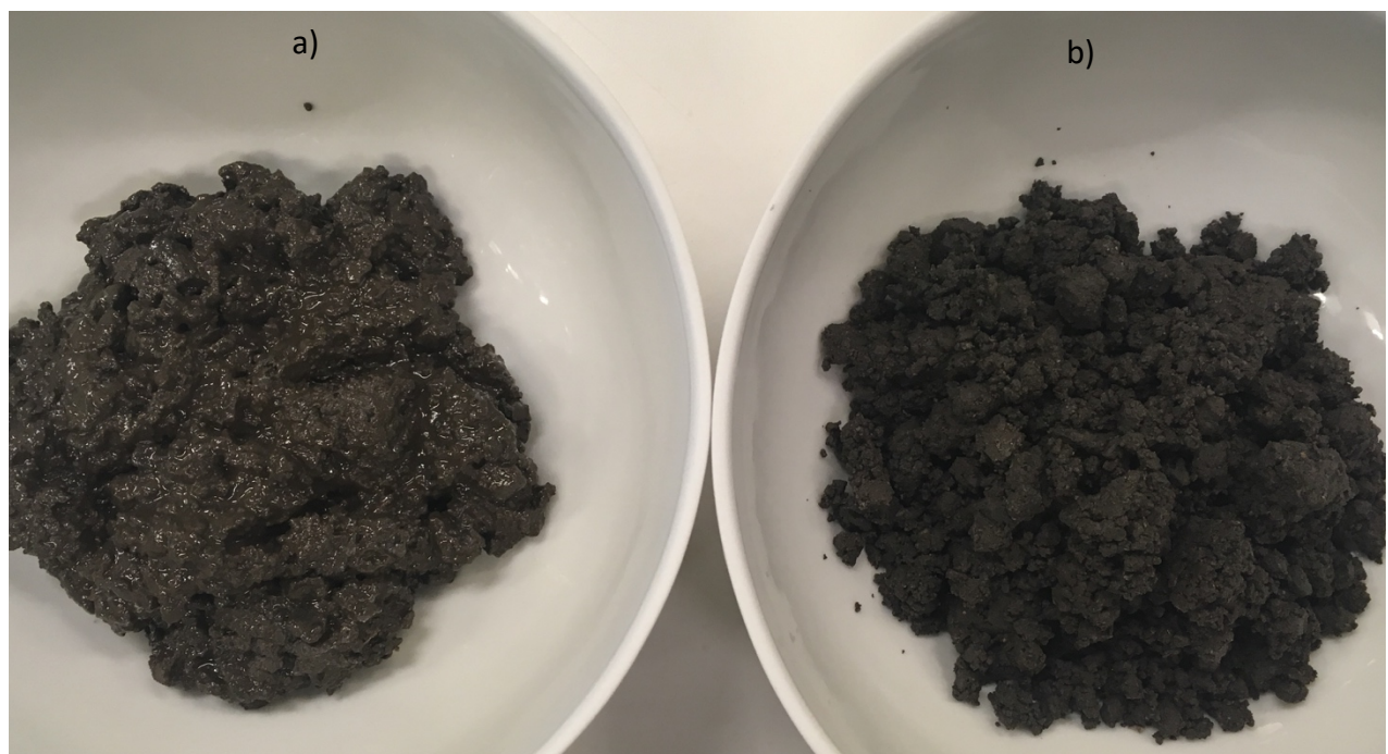
Figure 60: Structure of raw and centrifuged cuttings
