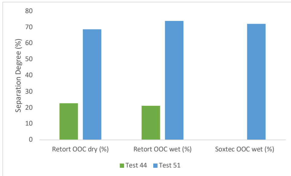
Figure 59: Separation degree obtained in when alternating power density in Experiment 6
