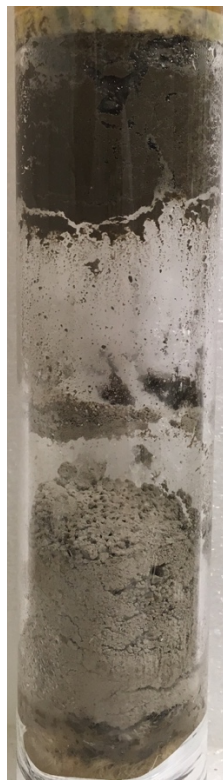
Figure 35: A part of the sample pushed up due to solid entrainment
