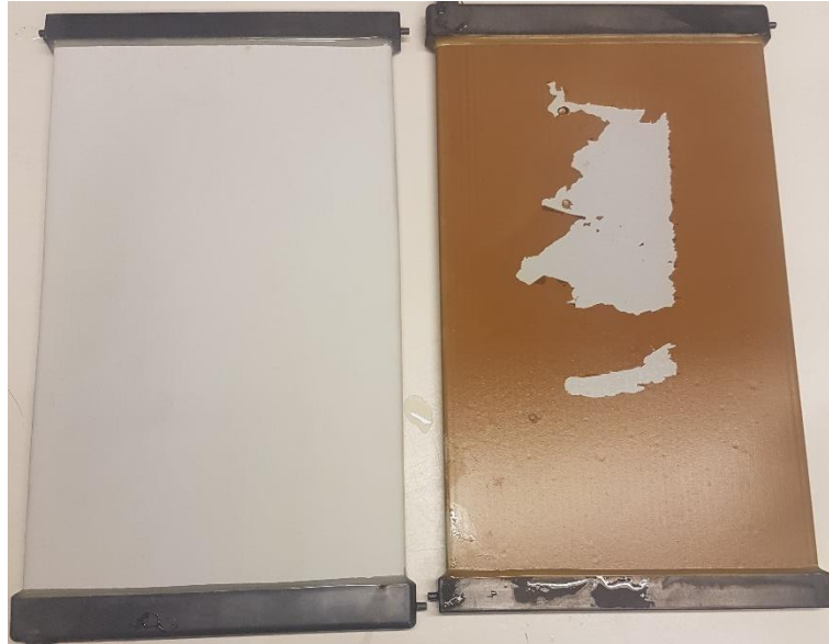
Figure 52: Clean membrane (left) and membrane with fouling layer, after hydraulic backwash
