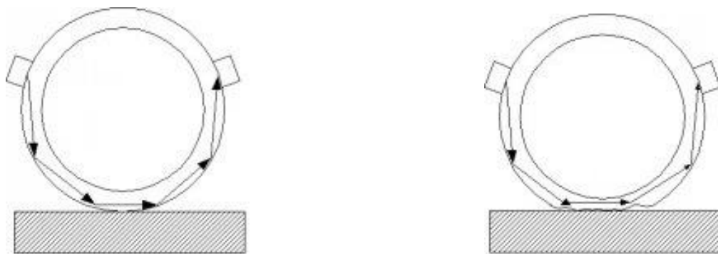
Figure 8-6 EMAT inspection without piping clamp
