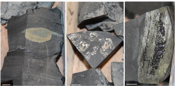
**Fig. 40** Left photo: A lense shaped pyrite nodule exhibiting zonation from well 7120/2-2, depth 2640.50. Middle photo: The bivalve fossils observed in well 7120/2-2–2642.50 show that pyrite has acted as a replacement mineral in the fossilized shell. Right photo: Woody material from well 7120/2-2, depth. The white line the left lower corner of the photos represents 1 cm.
