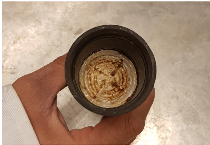
Figure 5.5: Picture of the inlet of core SK1, still in the rubber sleeve, after being subjected several PV of sulfuric acid and high temperatures.
