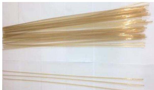
Figure 3.1: Polymers with chemical tracers incorporated (Mehdiyev, 2018).
