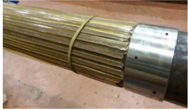
Figure 3.2: Polymer strips installed along the completion of the well pipe (Gashimov et al., 2017).
