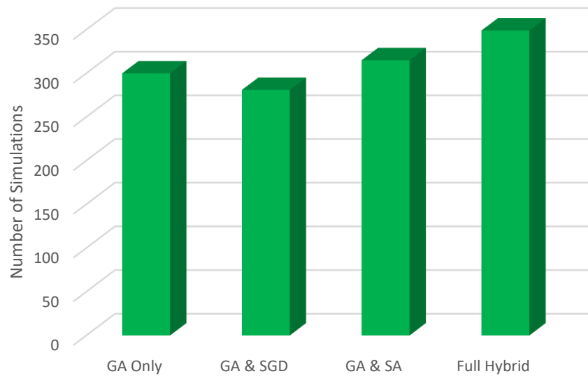
Figure 4. 22 Number of simulations ran in different optimization algorithms for the problem of moderate drilling cost
