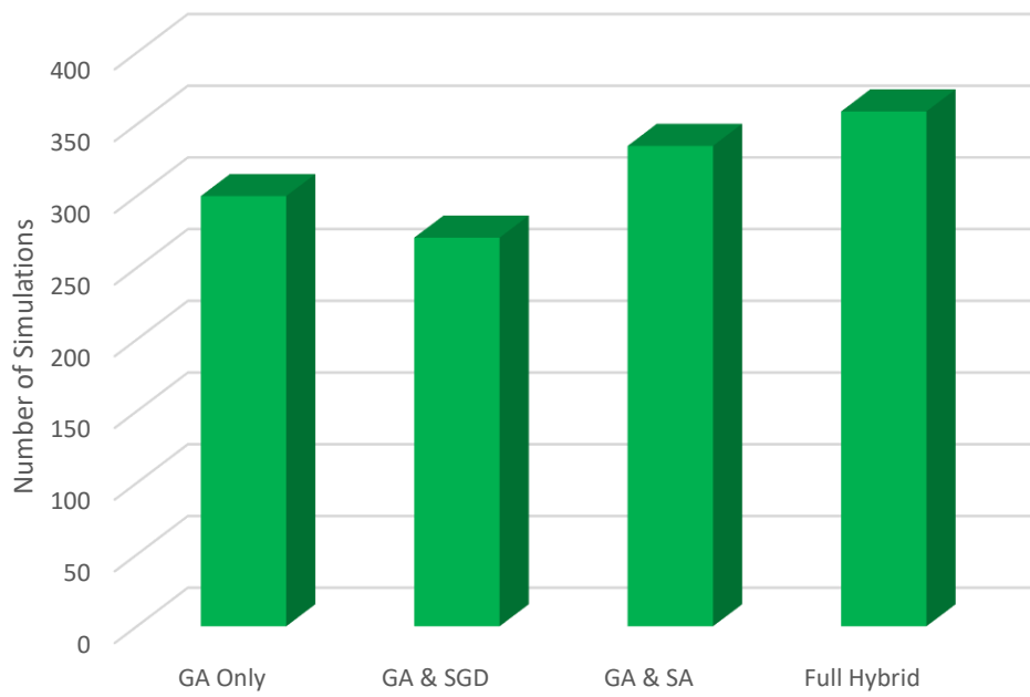
Figure 4. 24 Number of simulations ran in different optimization algorithms for the problem of costly drilling
