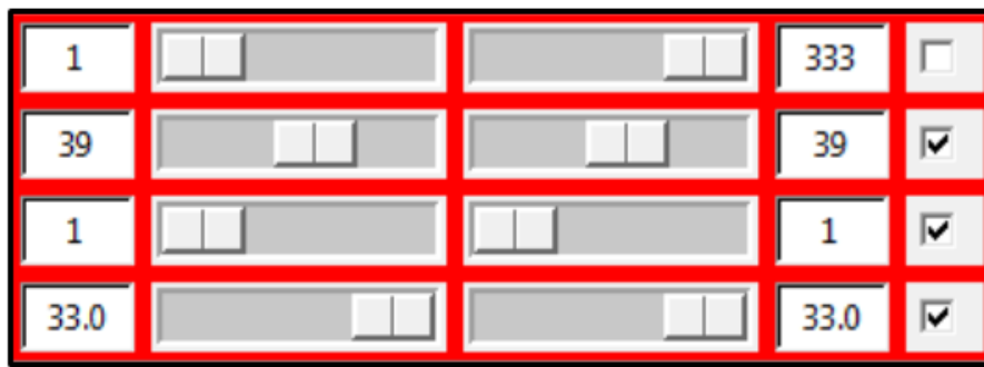
Figure 2.5: Data selection tool that, starting from the top, is used to select a range of grid cell i , j and k values, in addition to a range of timestep values. This controls which grid cell data is available for visualization of 1D, 2D or 3D simulation data. The checkmarks to the right sets the value of each respective slider equal to each other. Either slider could then be used to alter that singular value.
