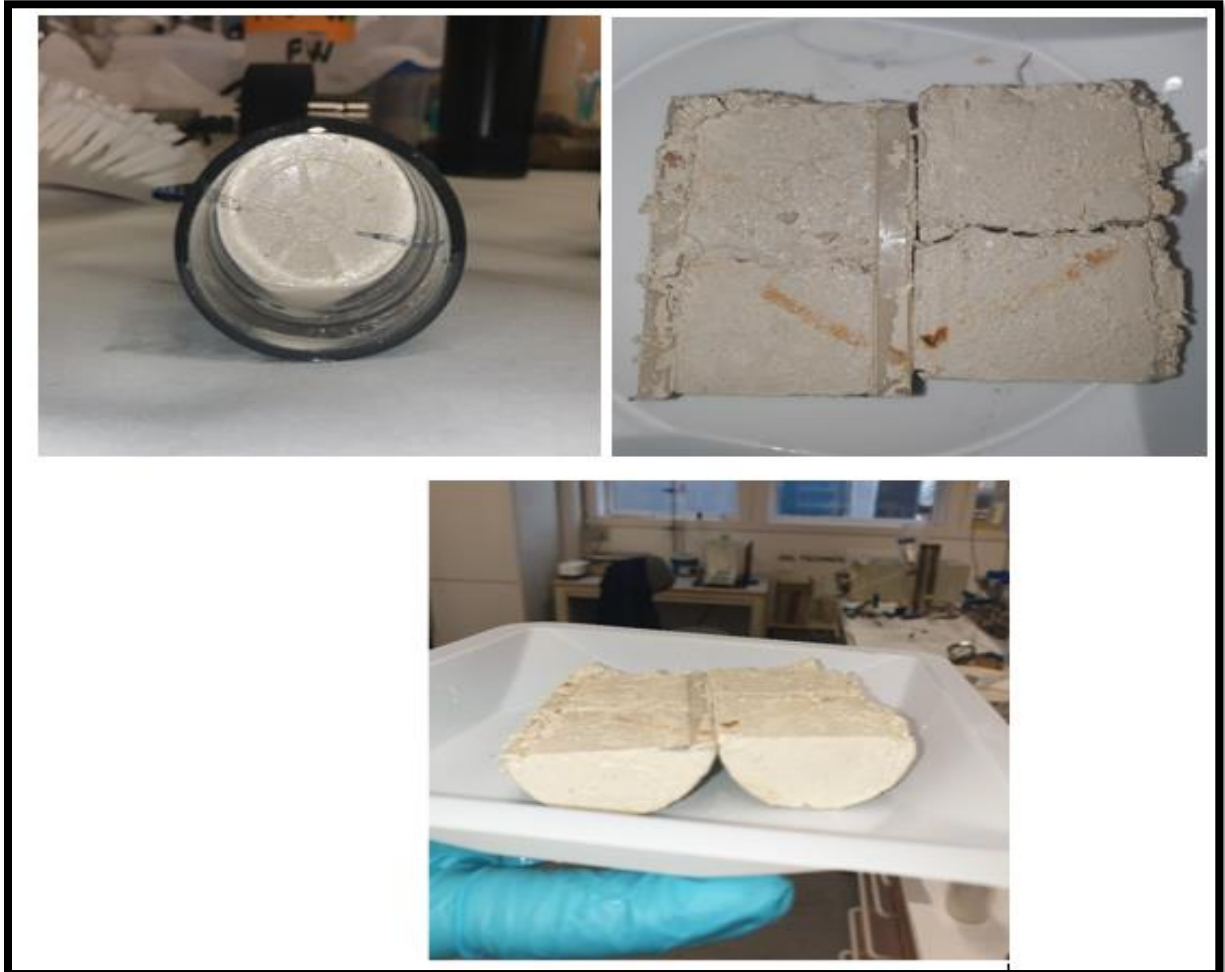
Figure 5.15: collapsed fracture aperture, (a) before removing the core plug from the core sleeve, (b and c) upon removal and closer inspection of the core plug
