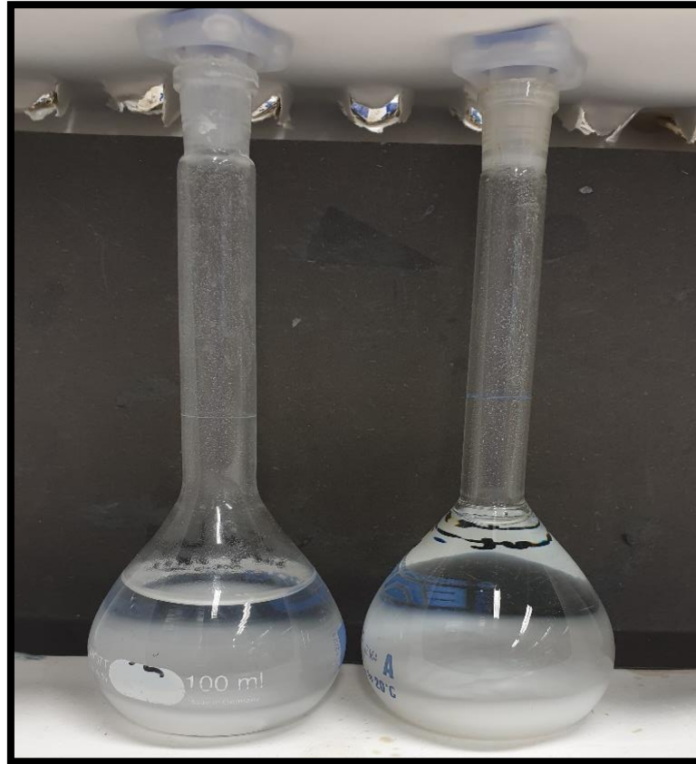
Figure 5.6: Flocculation of laponite when prepared in seawater
