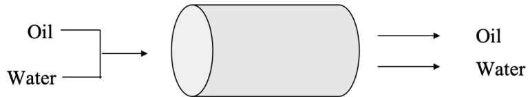
Figure 5.1 Illustration of measuring relative permeability for water and oil at (a) Unsteady-state method and (b) Steady-state method. Redrawn after Lucia (2007)
