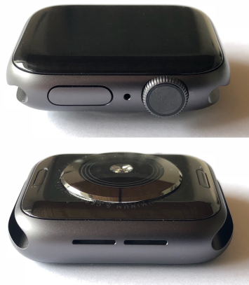
Figure 2.4: The Apple watch series 4 with one electrode on the back, and one electrode at the crown 3 [4].
