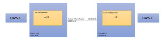
Figure 3.3: Lab setup without core network
