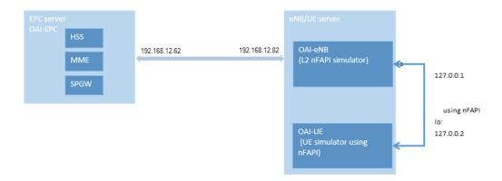
Figure 3.6: Lab setup using nFAPI [27]
