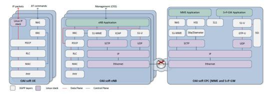
Figure 3.1: OpenAirInterface LTE software stack [20]
