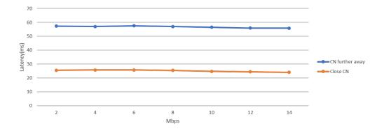
Figure 4.22: Latency in milliseconds at Tampnet's lab
