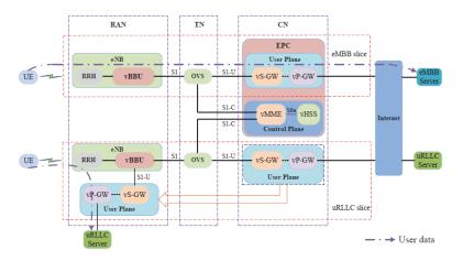
Figure 2.7: Slicing architecture from OAI-based End-to-End Network Slicing [13]
