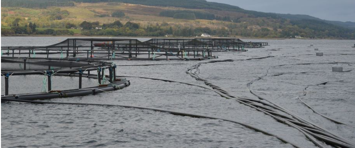
Figure 2.8: Feeding tubes from a feeding barge going to multiple fish cages at a Scottish aquaculture facility [18].
