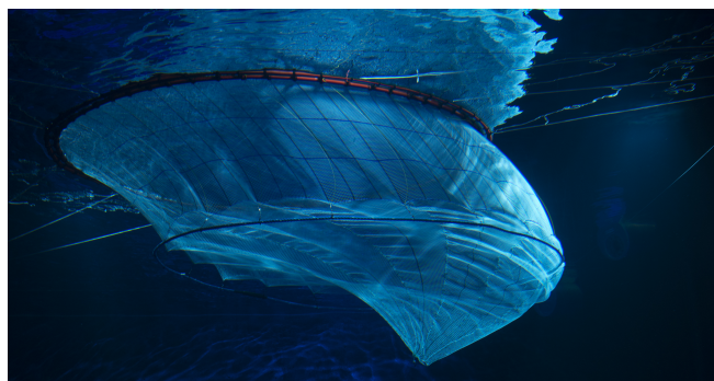
Figure 4.1: A cylindrical fish cage with a conical bottom section, manufactured by Egersund Net AS, here seen undergoing steady current tests [24].
