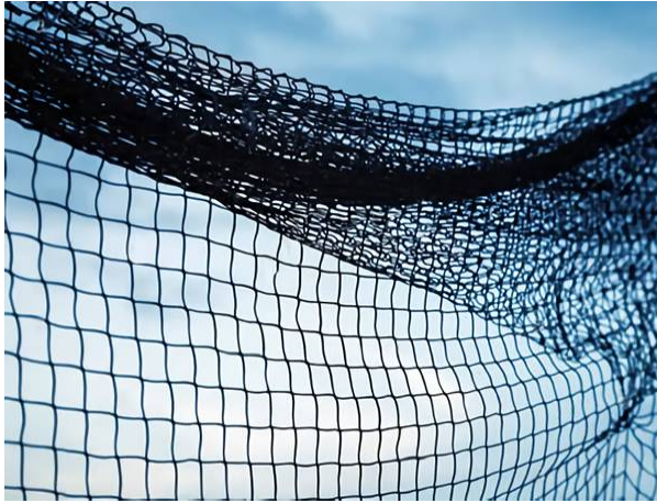
(a) Knotless fishing net with square meshes (Source: GuangTong Plastic Netting)
