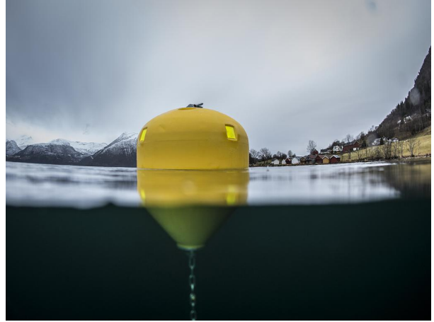
(b) Mooring buoy floating in a near shore fish farm (Source: Polyform AS)
