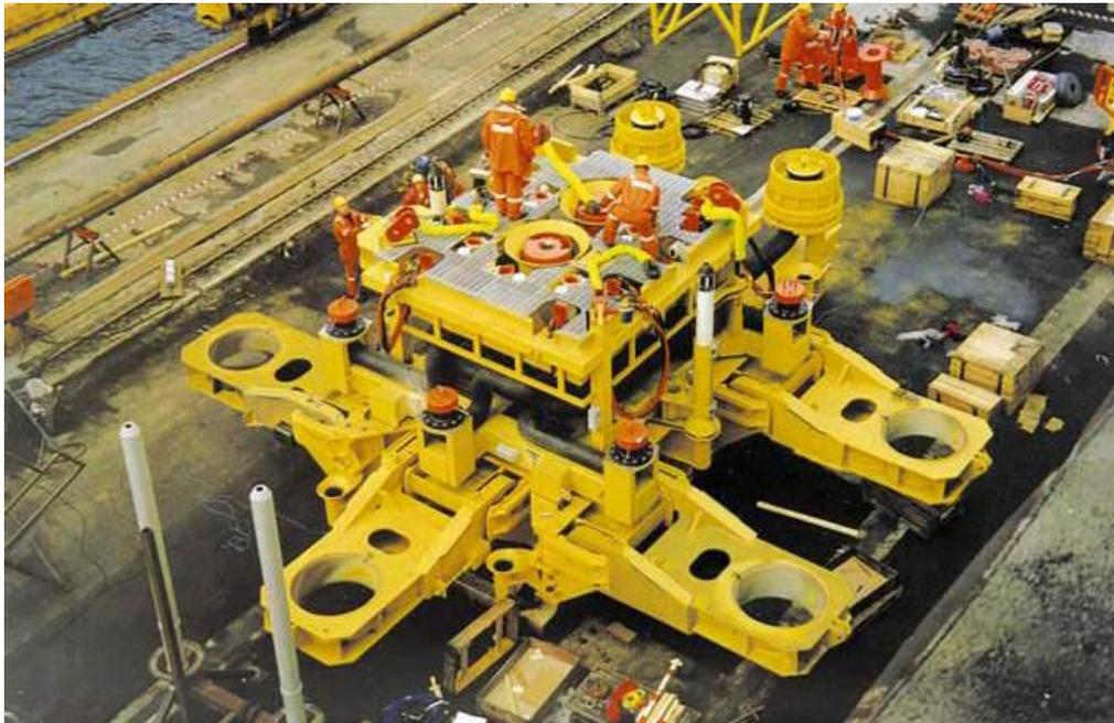
**Figure 19. Five slot subsea template [42].**
