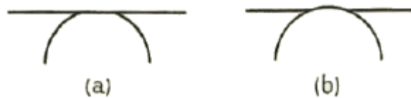
Figure 3:22: Deformation of asperities: (a) hemispherical asperity deformed by a flat surface. (b) flat surface deformed by a hemisphere. The deformation process is similar in both cases [29].
