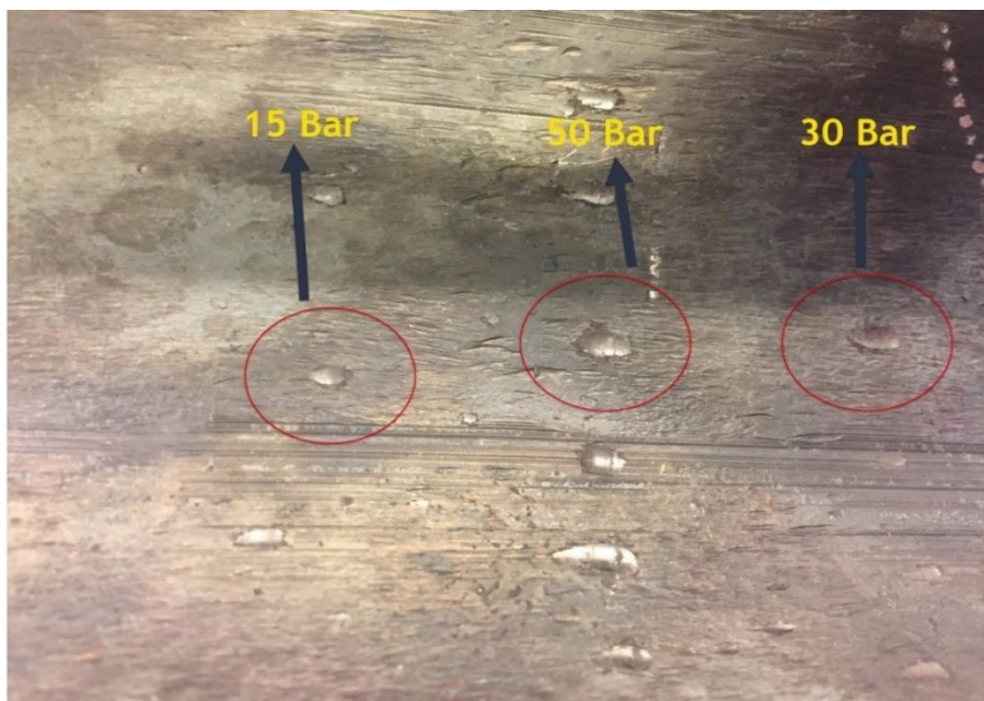
Figure 8:7: Picture of spherical deformation on the pipeline wall with Set-Pressure of 15,30 and 50 bar when used a cone of 3-degree angle alloyed with Calmax.
