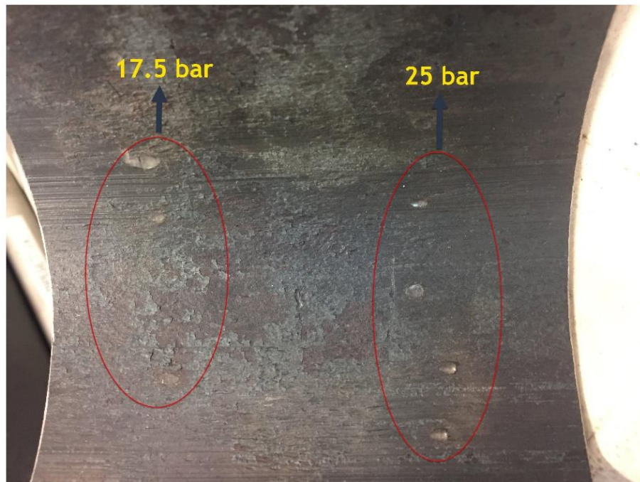
Figure 8:9: Picture of spherical deformation on the pipeline wall with Set-Pressure of 17,5 and 25 bar when used a cone of 4-degree angle alloyed with Calmax.
