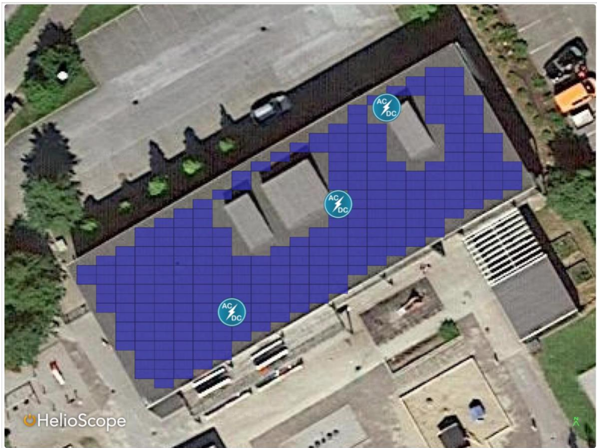
Figure 4.1 Solar PV arrangement at Barnebage roof
