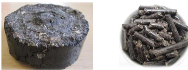
Figure 2.12 The form of bio-coal: briquette (left) and pellets (right) (Agar and Gil, 2013)
