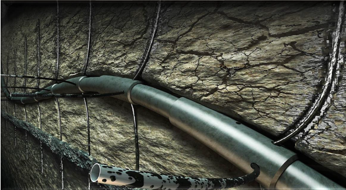
Figure 1.1: Illustration of Fishbones technology [2]. Multiple subs attached to the main pipeline with three needles coming out creating laterals.
