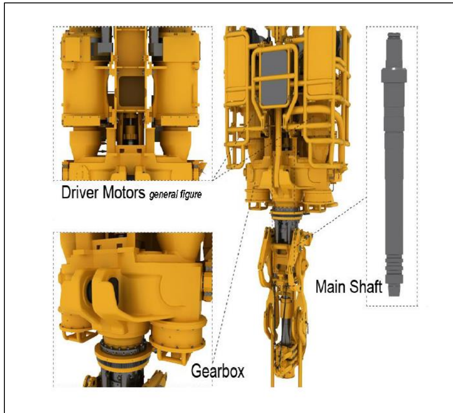
Figure 5-1: Illustration showing the upper part of the HPS-03 1000T top drive with its drive system
