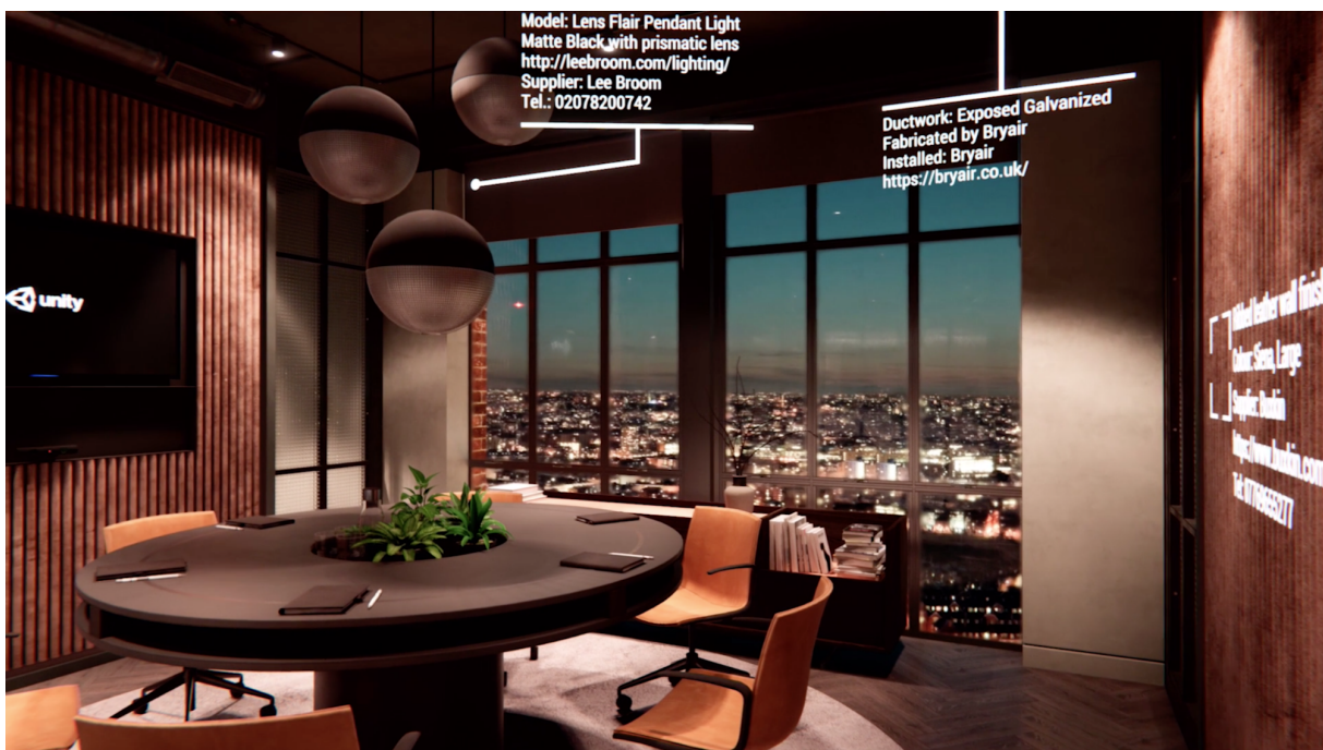
Figure 3.16: Screenshot from a video illustrating the potential of Unity. The figure shows the user in VR being able to directly access information about items in the model [74].
