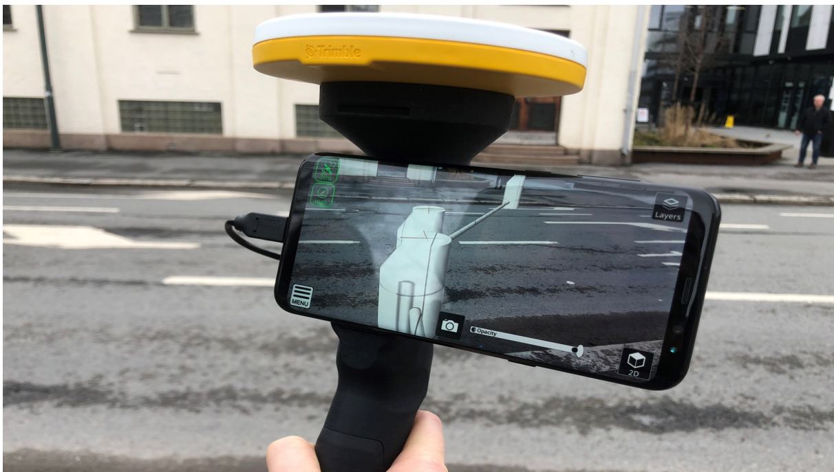
Figure 3.17: Demonstration of Trimble SiteVision on a mobile device with the GNSS device. Picture provided by Skanska.
