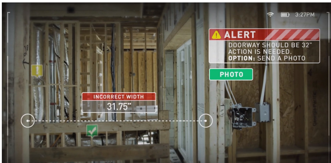
Figure 5.4: Screenshot from a concept video demonstrating how AR could be used for quality assurance [105].
