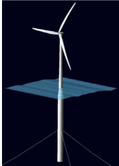
Figure 3.1: Illustration of the 5 MW NREL wind turbine on the OC3-Hywind spar-buoy FOWT
