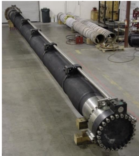
Figure 1.2 Example Composite Drilling Riser (Pangaea Drilling, 2019)
