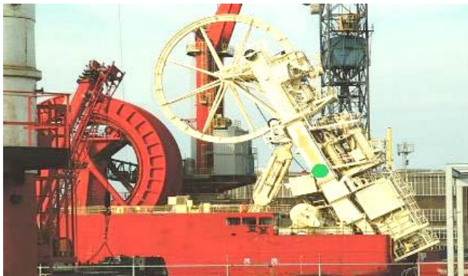
Figure 5. 3: Straightener equipment in a reel-lay vessel. (Wartsila Encyclopedia of Marine Technology, 2016)
