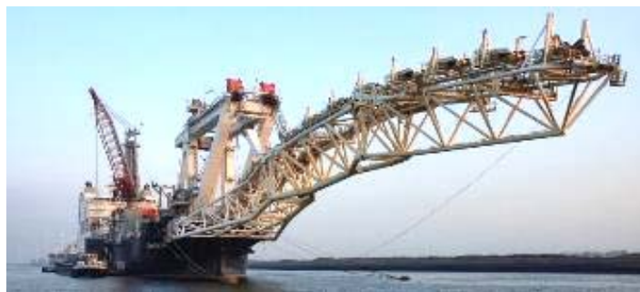
Figure 4. 2: S-lay installation vessel Audacia, Allseas Group – Length of 225m. (All seas group, 2015)
