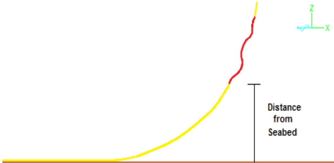
Figure 7. 25: Illustration of parameter distance from seabed to RC section (No real curvature in section)
