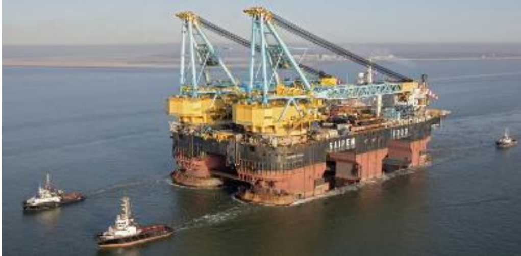
Figure 4. 5: Saipem 7000. Semi-submersible crane and pipe laying vessel. (Saipem, 2010)
