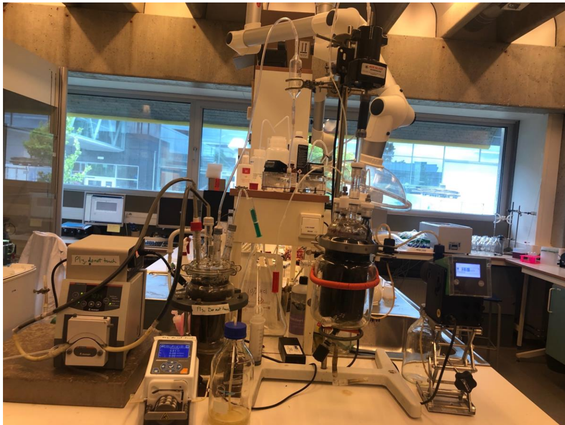
Figure A.1 Photo of Experimental Set Up of CFSTR, RI on The Right side and RII on the Left Side of The Picture
