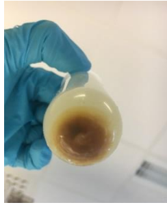
Figure 3.6: Final pellet after the last centrifugation step at 26000 x g in the mitochondrial preparation from beef liver.
