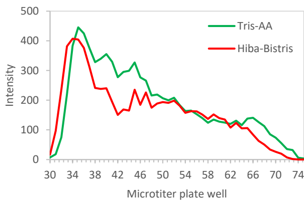
Figure 23. Fluorescence readings when exciting at 435 nm and emission at 680 nm. Fractions 30 – 75 are shown from the FFE separation of solubilised stroma lamellae membrane complexes from freshly isolated chloroplasts of A. thaliana WT-col. Different buffer systems were compared, 10 mM Tris - Acetic acid pH range 5 - pH 7 (red), and Hiba – Bistris (green). Intensity values times 10 6 .
