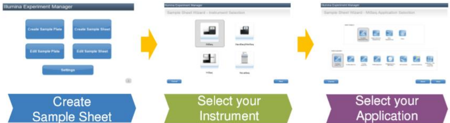
Figure 18: The layout of the steps to create a sample sheet in Illumina sequencing systems [96].
