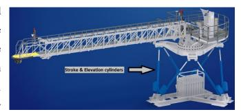
Figure 17 - Stroke & Elevation cylinders for gangway bride (Ampelmann, 2019)
