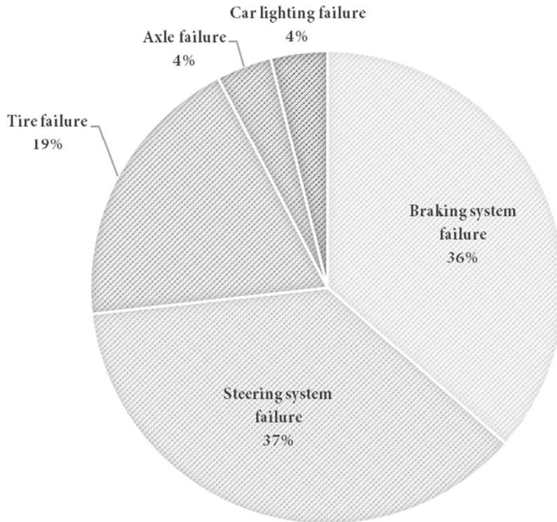
Figure 12 Mechanical failure car crash cause
