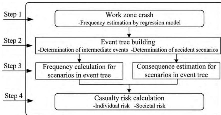
Figure 3 Flowchart for QRA model formulation (Meng et al., 2010)
