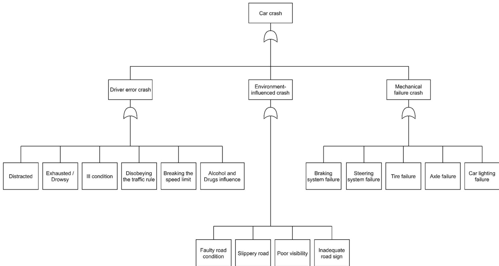
Figure 6 Fault tree model for Car crash
