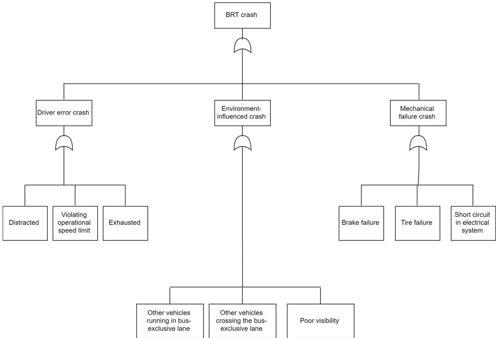
Figure 29 Fault tree model for Bus Rapid Transi (BRT) crash
