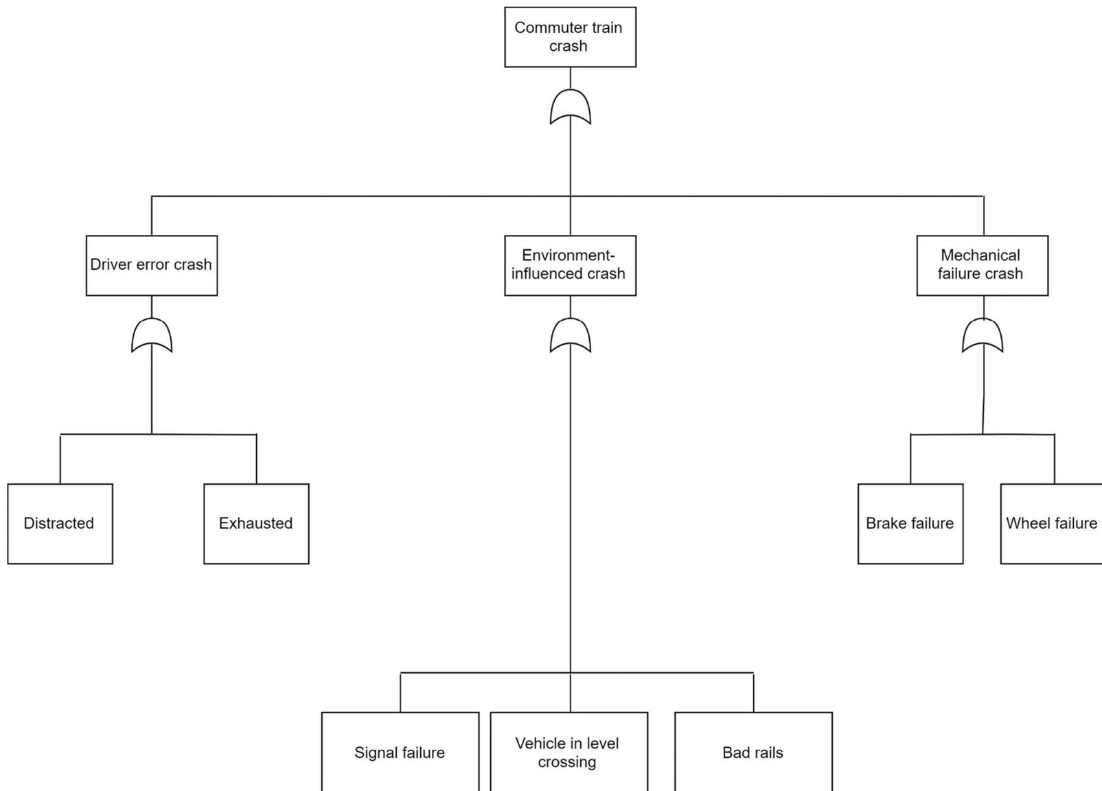
Figure 36 Fault tree model for train crash
