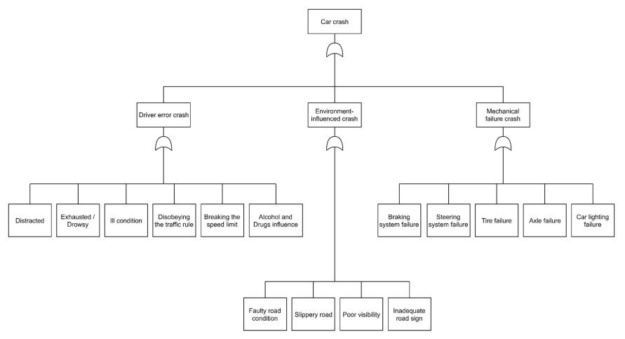
Figure 6 Fault tree model for Car crash
