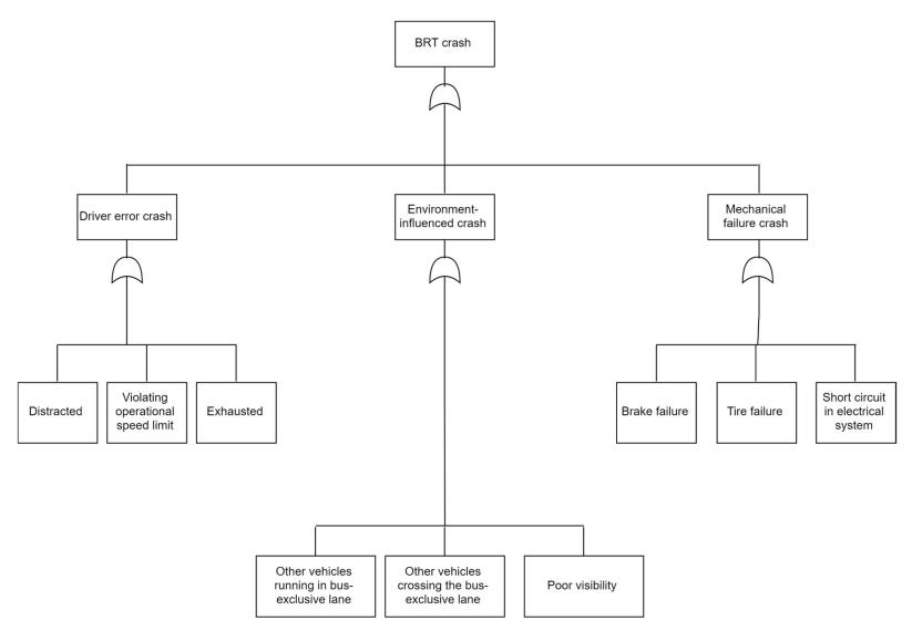
Figure 29 Fault tree model for Bus Rapid Transi (BRT) crash
