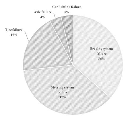
Figure 12 Mechanical failure car crash cause
