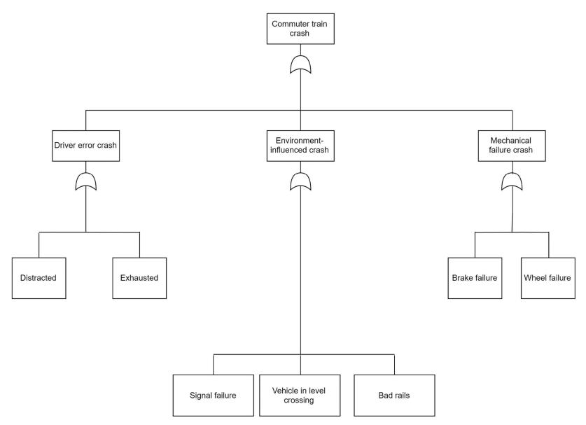
Figure 36 Fault tree model for train crash
