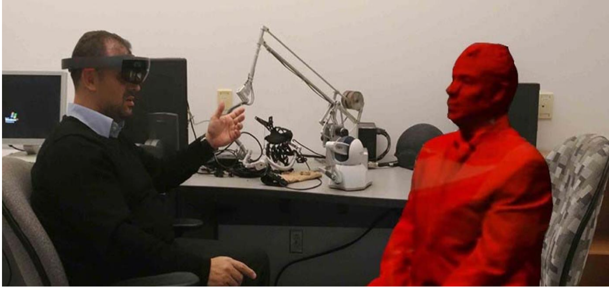
FIGURE 13 A SUBJECT INTERACTING WITH THE HOLOGRAPHIC REPRESENTATION OF HIS DIGITAL TWIN, WITH REFERENCE TO (SADDIK, 2018, P. 89).
