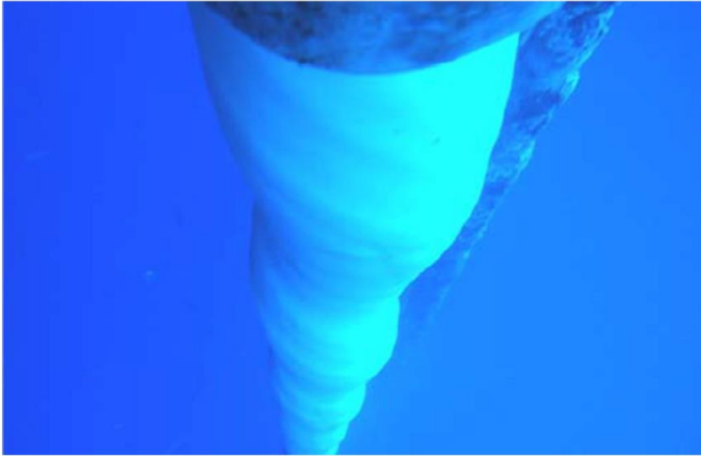
Figure 55 Shows torsion at the top of a riser due to ruptured armour wires[52]
