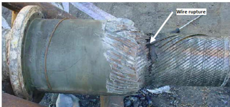
Figure 53 Rupture of tensile armour wire due to fatigue [52].
