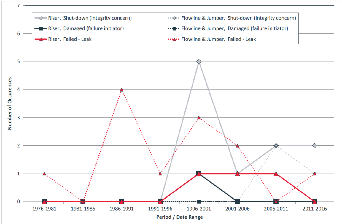
Figure 13 Showing the damage and failure timeline for internal pressure sheath ageing [2].
