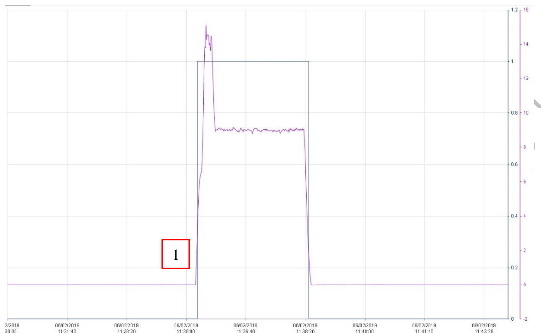
Figure 4. Deluge release – measured pressure and digital response when alarm limit is triggered
