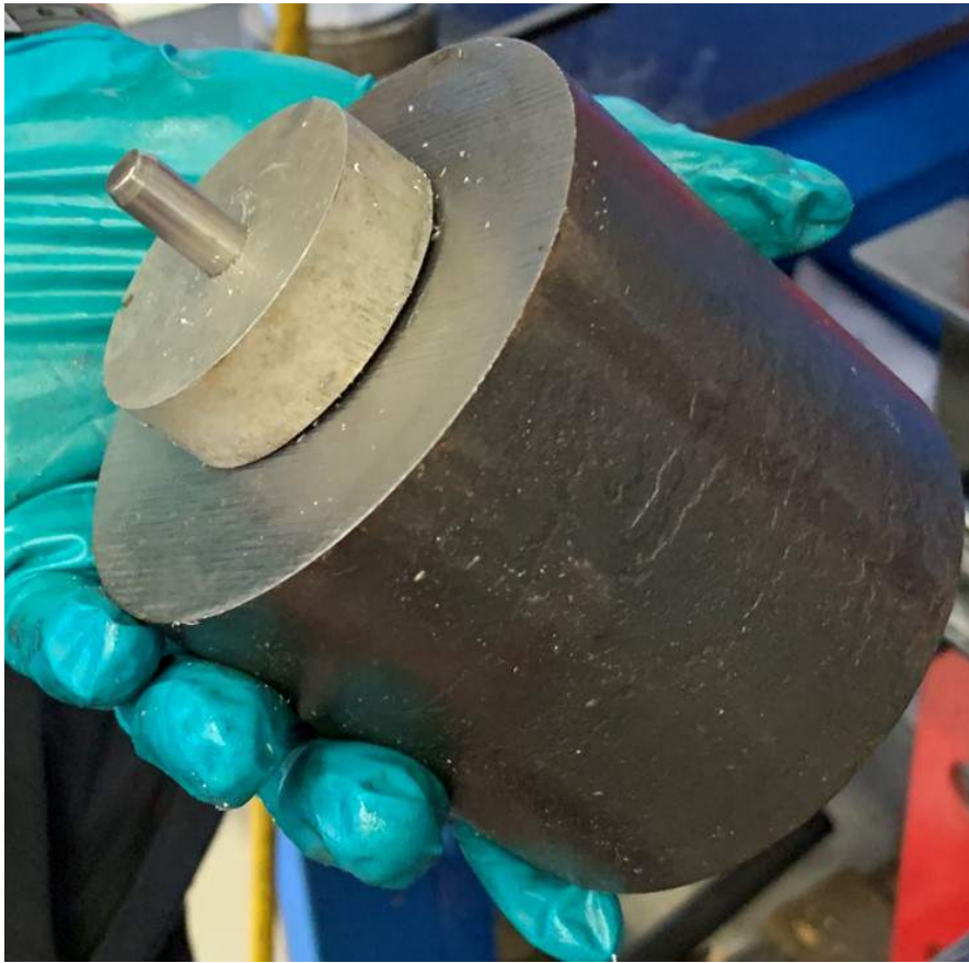
Figure 36: Parallel pin placed in steel bolt for guidance.
