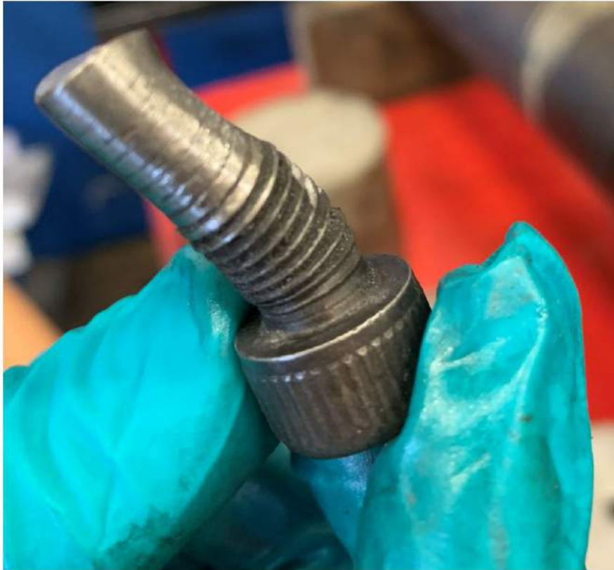
Figure 34: M12 bolt deflected after punch attempt.
