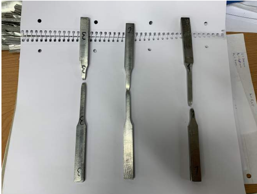
Figure 63: All test specimina after tensile testing.
