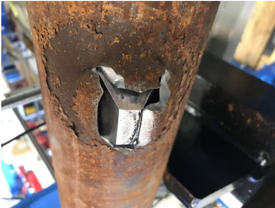
Figure 60: Punch pressed all through a casing.
