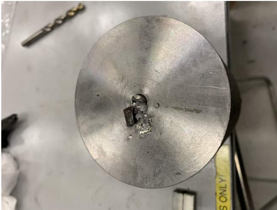
Figure 37: Shows broken parallel pin after punching.
