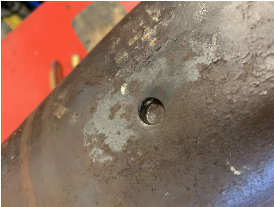
Figure 38: Indentation in casing from parallel pin punching.
