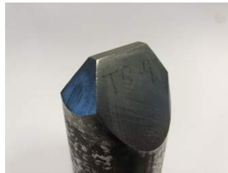
(b) Minor chipping.
