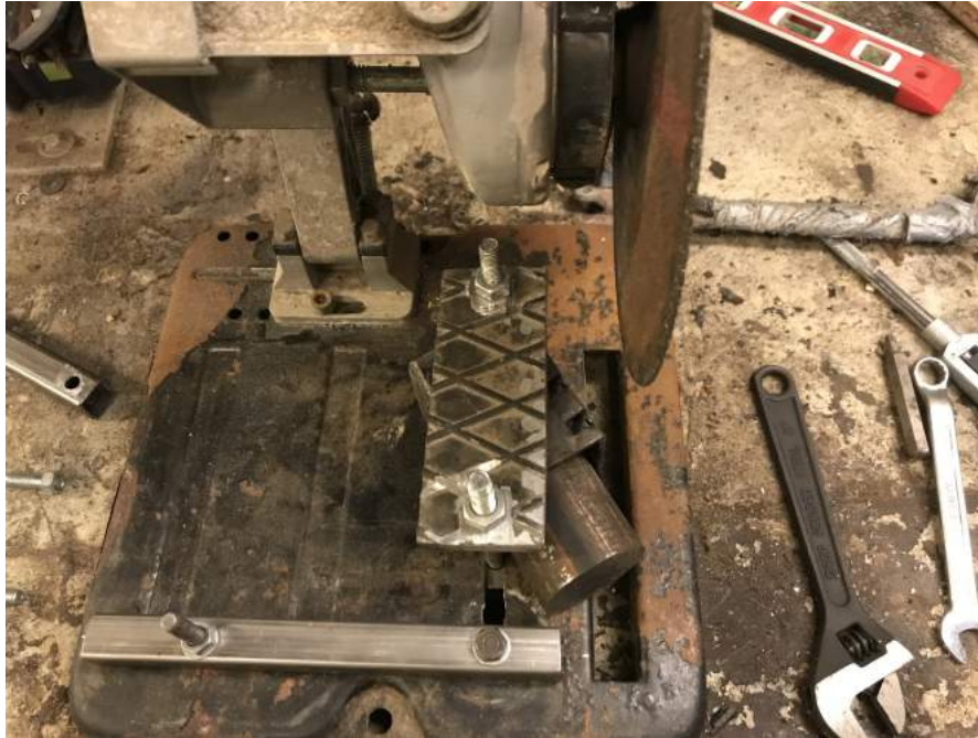
Figure 41: Punch in production, fastened at an given angle in an angle grinder jig.
