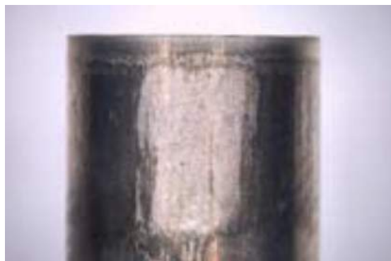
Figure 11: Example of galling wear [59].
