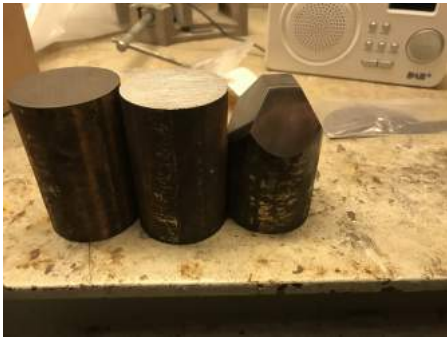
(a) 4145 bolt before production and finished (b) All punches after production ready for testing.
