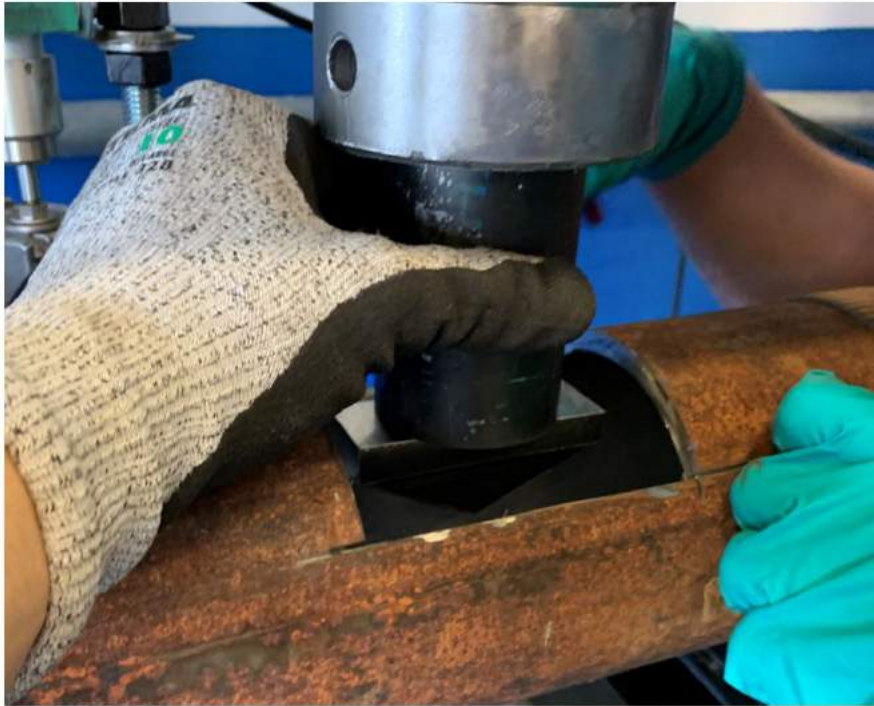
Figure 54: Puncher mounted in the hydraulic press.
