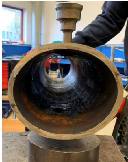
Figure 58: Casing after punching, note the deflection in the casing.
