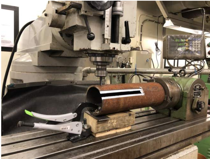
Figure 46: Casing secured to rotary table during machining.
