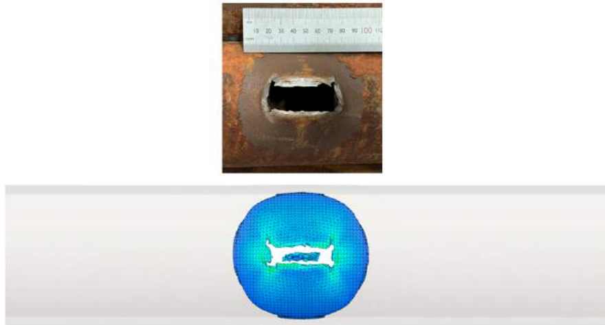
Figure 88: TB-4 comparison of area above yield threshold in test result and FEA result.
