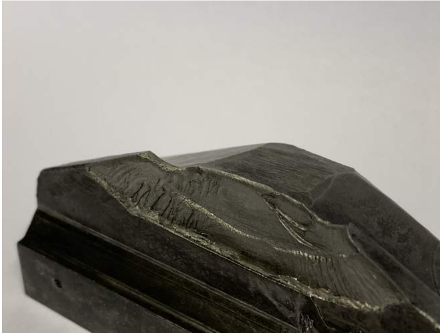
Figure 104: Gross fracture of prototype.
