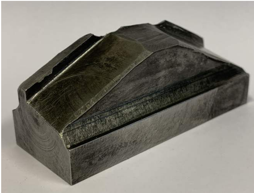
Figure 105: Plastic deformation of face and vertex of lifting flank.
