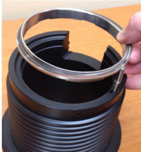
Figure 2.23. Version 2 design as being field removable and replaceable (NOVMaterial)
