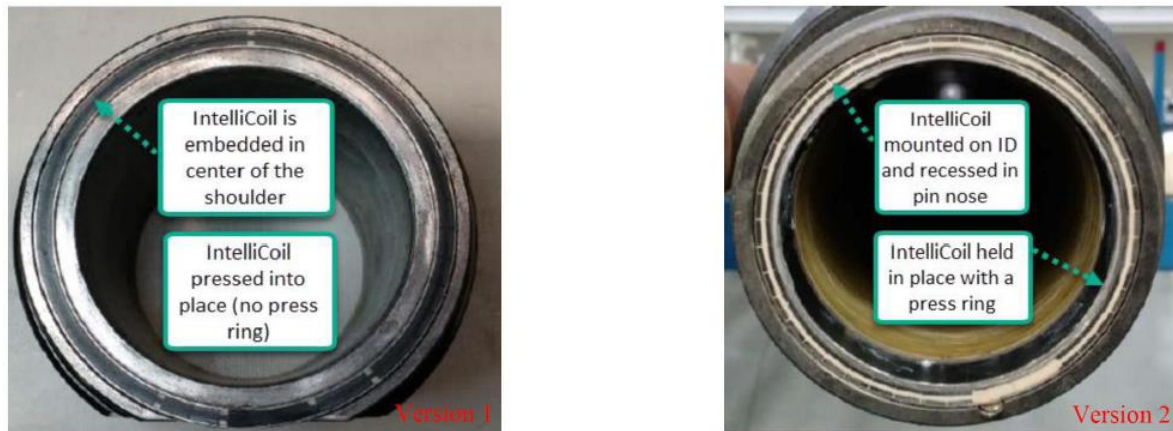
Figure 2.22. Wired pipe version 1 and version 2 coil mounted in the center of the shoulder of the PIN(NOVMaterial)
