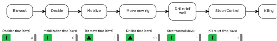
**Figure 4.11:** *The different phases of a relief well process, with corresponding estimated duration.*
