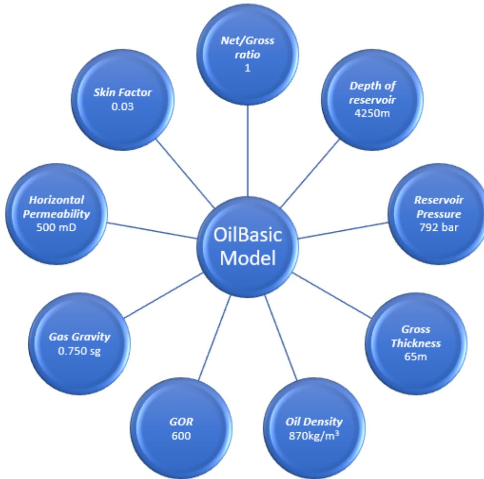
**Figure 4.5:** Reservoir zone properties with the use of OilBasic model.
