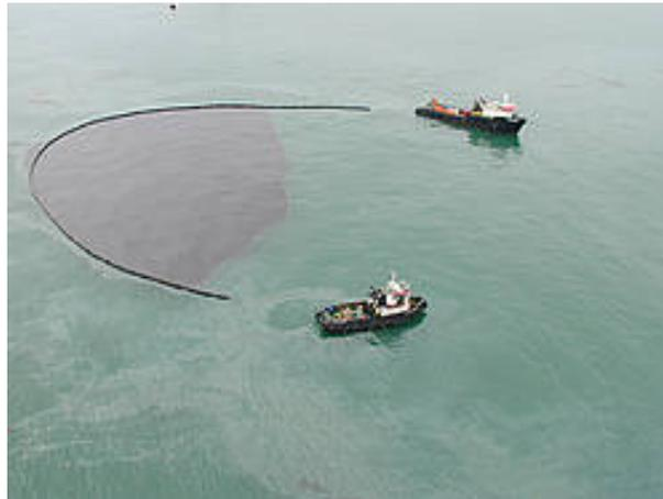
**Figure 2.4:** *Boom deployed in an U configuration between two vessels to capture oil (ITOPF, 2018).*
