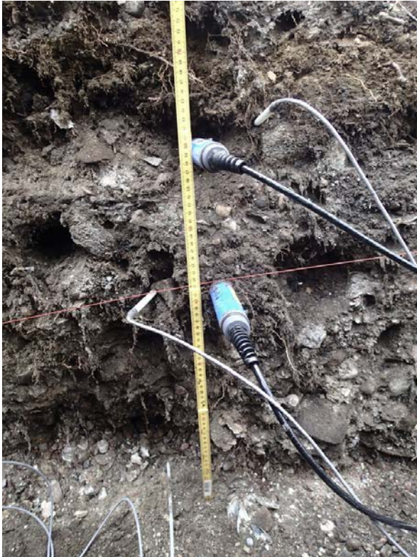
Figure 30: Probe set 2. White probes: redox/temperature. Blue probes: moisture/ temperature. Photo: MVH Consult.
