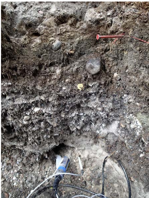
Figure 32: Probe 1.5 (set 4) in the Northern corner. Blue probe is the moisture/temperature sensor installed by Bioforsk/NIBIO. Photo: MVH Consult.
