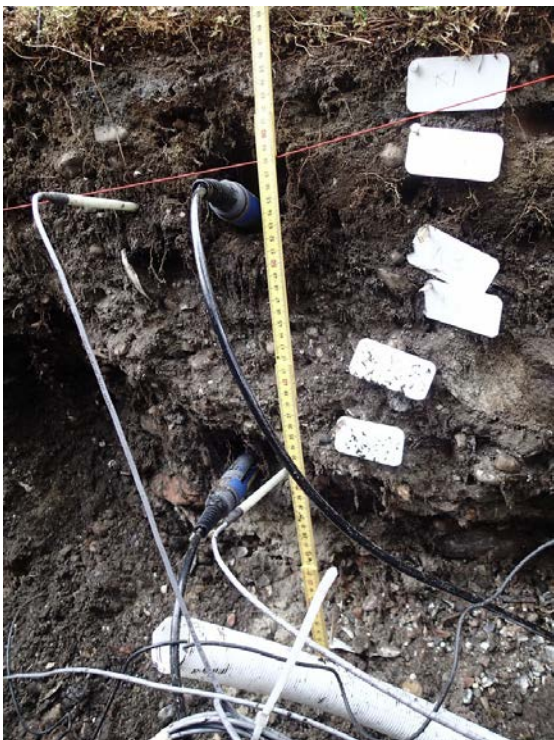
Figure 31: Profile set 3. Red marker line is artificial 0. White probes: redox/temperature. Blue probes: moisture/temperature. Photo: MVH Consult.
