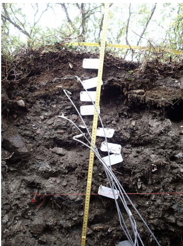
Figure 29: Profile set 1 in Southern corner, probe 0.0 to 0.5. Note the very dry soil profile. Red line indicates artificial zero. Photo: MVH Consult.
