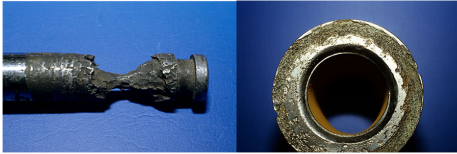
Figure 6 - Crevice corrosion on axle and flange [13] [14]
