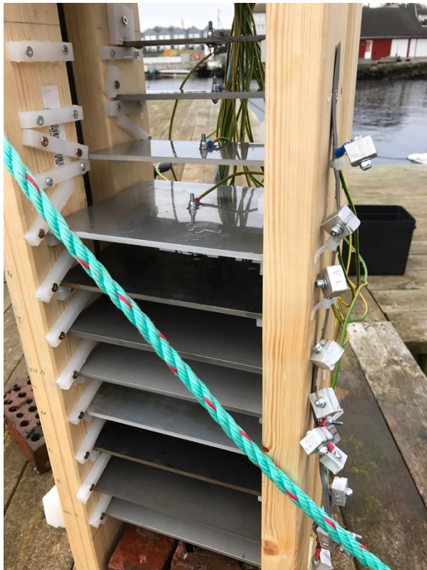
Figure 23 - Cathodes and anodes mounted on the buoy
