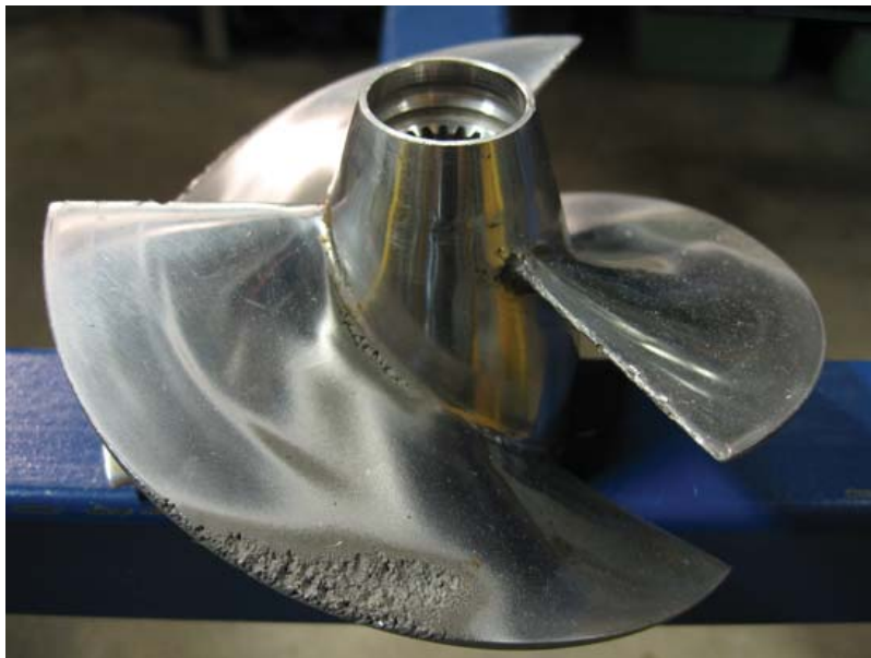
Figure 12 - Erosion corrosion caused by cavitation [20]
