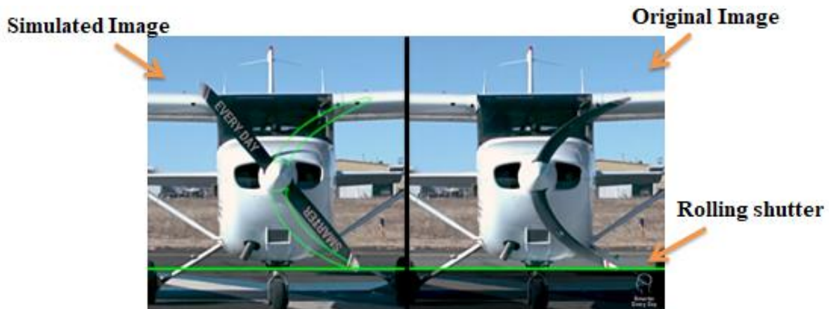
Figure 42: Effect of rolling shutter on moving propeller [37]
