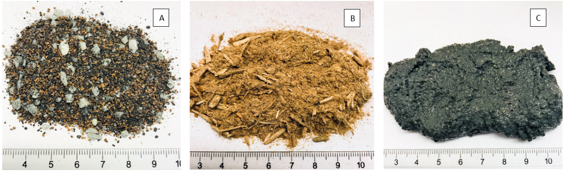
Figure 3.5: The three different lost circulation materials used in this experiment. A) ONS-mixture, B) StopLoss, C) QuartzPack
