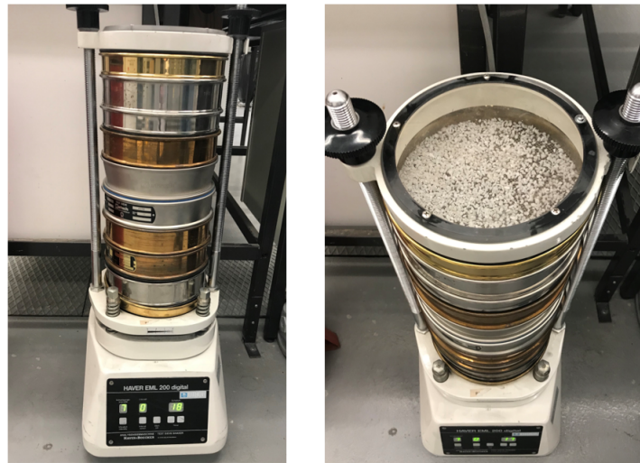
Figure 3.4: Test sieve shaker to determine the particle size distribution of LCM.
